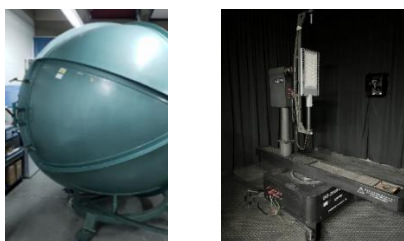
Figure 2: Ulbricht Integrating Sphere and Goniophotometer
