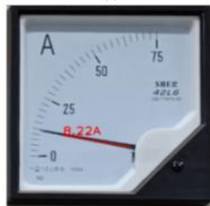
Figure 3. Example of inference from the reading of the ammeter needle. Source: (Zhang et al., 2023)
