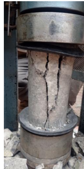
Figure 4. Specimen breakage in axial compression test
