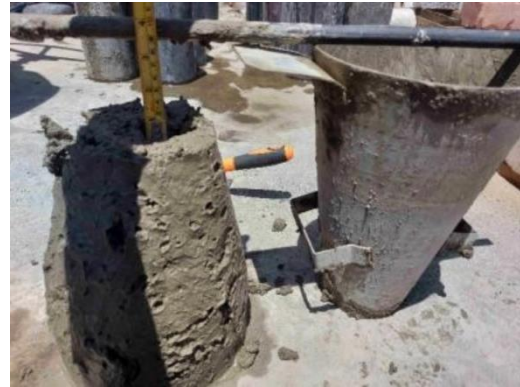
Figure 3. Slump test of concrete in fresh state
