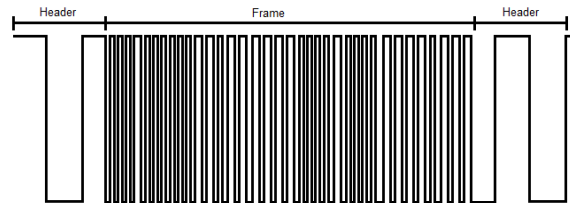
Figure 3. Logical sequence of 1s and 0s of the infrared signal to turn off the equipment.
