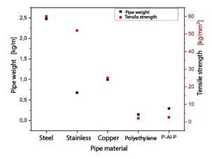
Figure 5. Factors for selecting LPG pipes. Adapted from [48]
