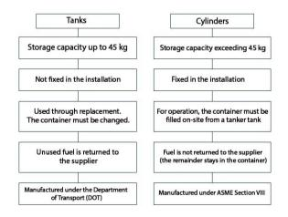
**Figure 2.** Differences between cylinders and tanks Adapted from [32, 33]
