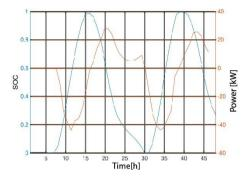
Figure 13. BESS usage cycle in 48 hours
