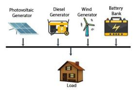
**Figure 8.** Diagram of the isolated microgrid based on ERNC
