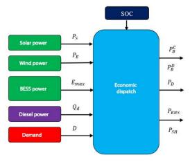
Figure 2. Block diagram used in economic dispatch
