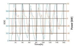
Figure 14. BESS usage cycle in 168 hours
