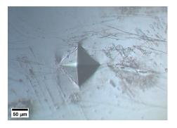
Figure 9. Microhardness evaluation of the 316L stainless steel processed by LPBF.
