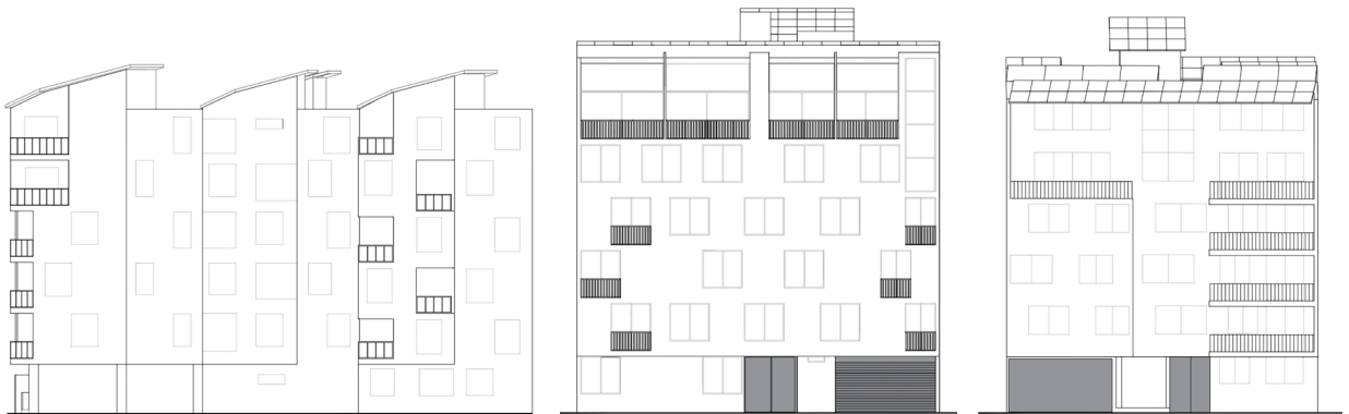
Figure 6: Classification according to the influence on the façade. a) sawn façades b) façades with interior slope overhangs, c) exterior projected slope façades, c) façades with exterior slope overhangs. Prepared by the authors on the basis of FAU-URP, Taller 9, 4th semester student's projects (2019-2023)
