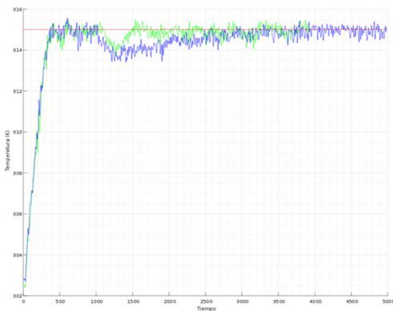
Figure 8. Experimental results comparing recovery time with and without fault compensation schema. With fault compensation represented by green curve. Without compensation represented by blue curve.
