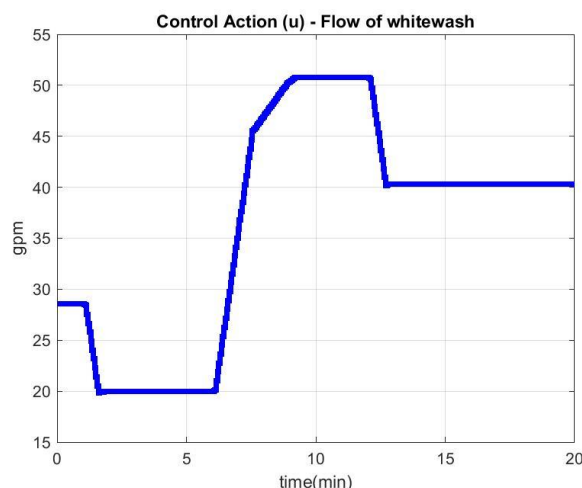
Figure 8. Time evolution of manipulated variable: flow of lime slurry.
